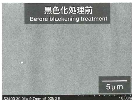
黒色化処理前後の表面SEM写真(×5,000) SEM image of surfaces plated before and after blackening treatment. (×5,000)
